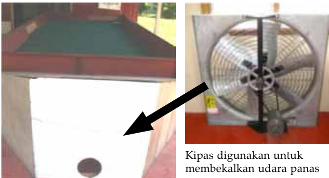
Gambar 1. Alat pengering daun lemon myrtle, withering trough
