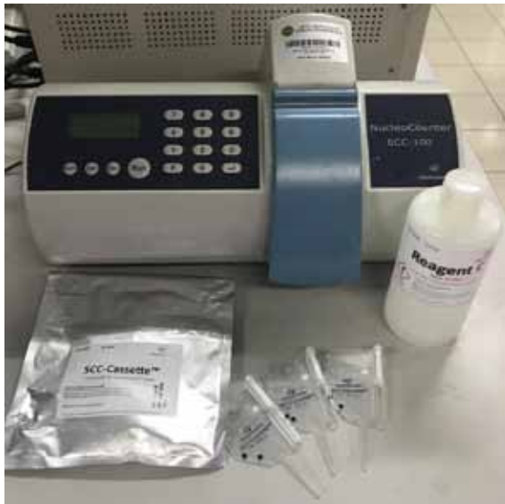
Gambar 4. Mesin NucleoCounter RSCC-100 TM berserta kaset dan Reagent C
