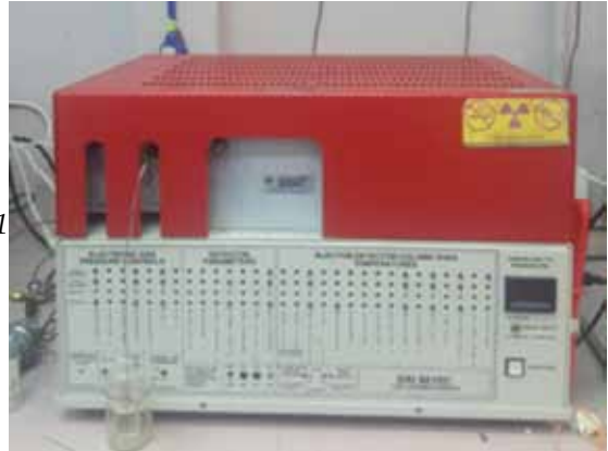
Gambar 12. Alat Chromatography Gas (GC)
