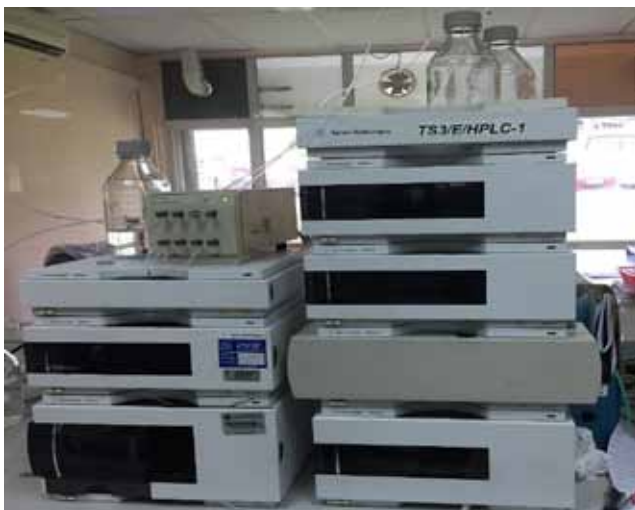
Gambar 3. Peralatan HPLC Agilent Technologies 1200 Series
