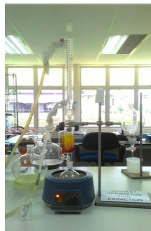
*Gambar 3. Radas soxhlet*
