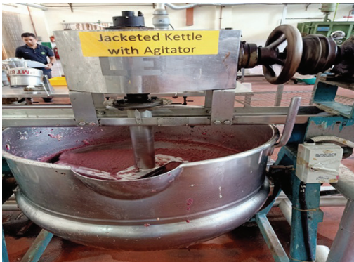
Gambar 3. Alat jacketed kettle bagi proses pengisaran bahan mentah
