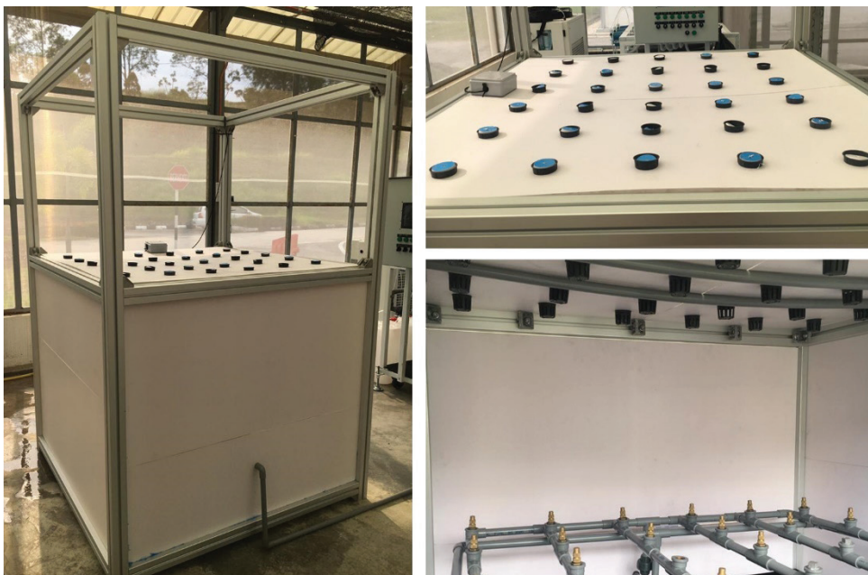
Gambar 2. Pemasangan lampu LED
